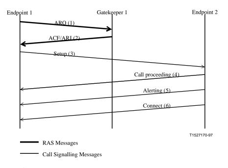
Figure 16/H.323 – Only calling endpoint registered – Direct call signalling
