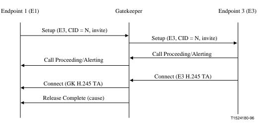
Figure 31/H.323 – Gatekeeper routed invite signalling
