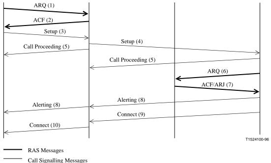
Figure 22/H.323 – Both endpoints registered – Routed/direct call signalling
