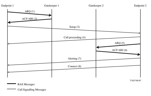
Figure 20/H.323 – Both endpoints registered – Both gatekeepers direct call signalling
