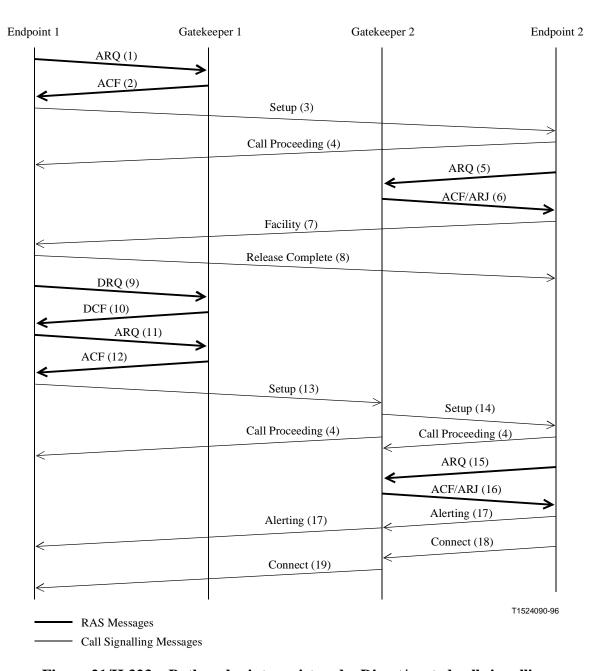
Figure 21/H.323 – Both endpoints registered – Direct/routed call signalling
