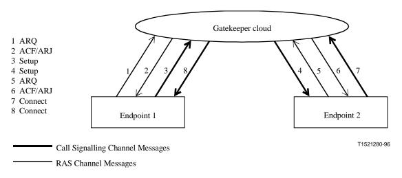
Figure 9/H.323 – Gatekeeper routed call signalling
