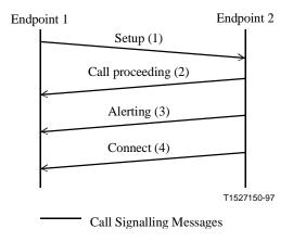
Figure 13/H.323 – Basic call setup, no Gatekeepers
