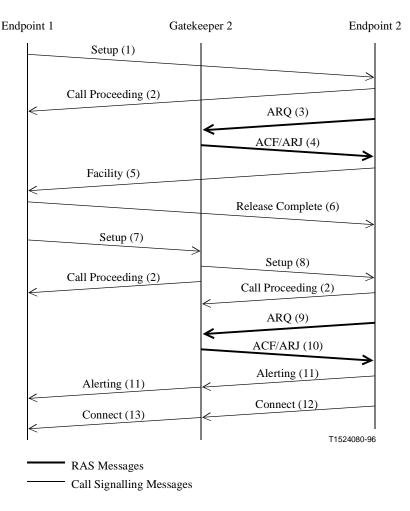
Figure 19/H.323 – Only called endpoint registered – Gatekeeper routed call signalling
