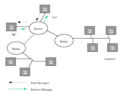
Figure II.1/H.323 – Resource reservation for a point-to-point connection
