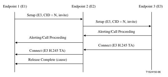
Figure 28/H.323 – Non-MC invite signalling
