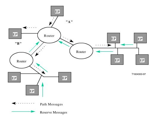
Figure II.2/H.323 – Resource reservation for a point-to-multipoint connection
