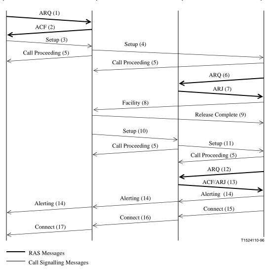
Figure 23/H.323 – Both endpoints registered – Both Gatekeepers routing call signalling
