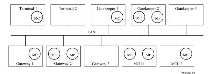
NOTE - Gateway, Gatekeeper and MCU can be a single device.
