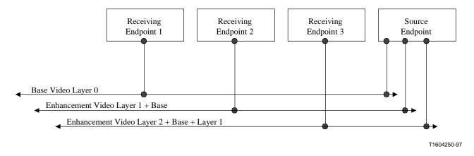
Figure B.3/H.323 – Endpoints attached to single Layer according to bandwidth
