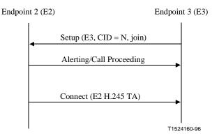
Figure 29/H.323 – MC join signalling
