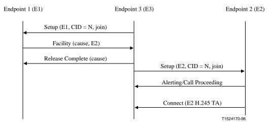
Figure 30/H.323 – Non-MC join signalling
