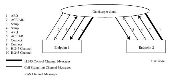
Figure 12/H.323 – Gatekeeper routed H.245 control
