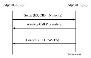
Figure 27/H.323 – MC invite signalling
