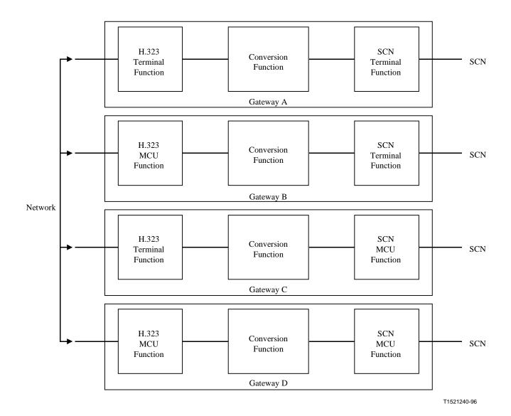
Figure 5/H.323 – H.323 gateway configurations
