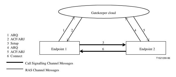
Figure 10/H.323 – Direct endpoint call signalling
