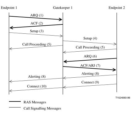
Figure 15/H.323 – Both endpoints registered, same Gatekeeper – Gatekeeper routed call signalling
