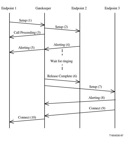
Figure III.1/H.323 – Example of user location using H.225/Q.931 signalling (RAS signalling not shown for clarity)
