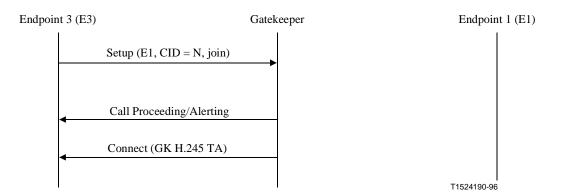
Figure 32/H.323 – Gatekeeper routed join signalling
