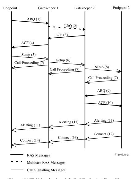
Figure 24/H.323 – Optional Called Endpoint Signalling
